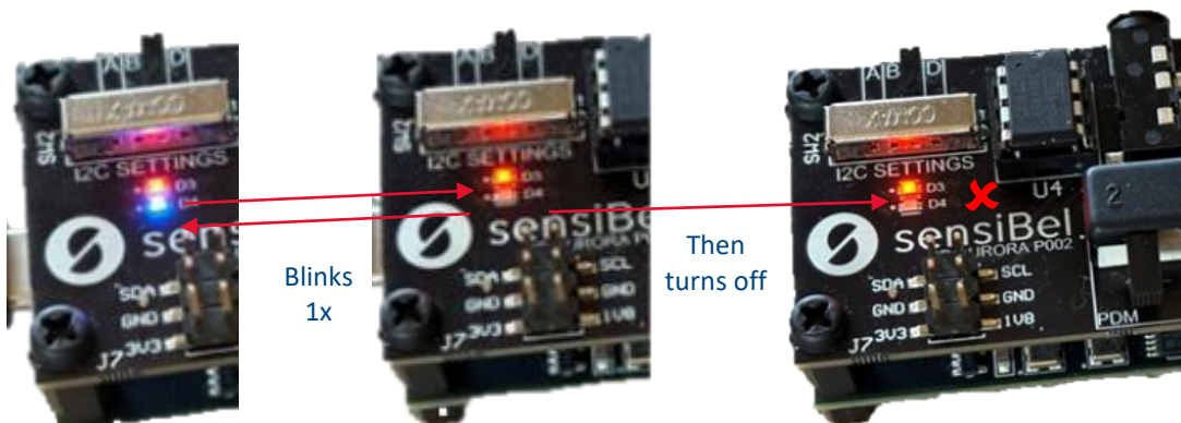
Figure 16. LED sequence for unsuccessful I2C write
