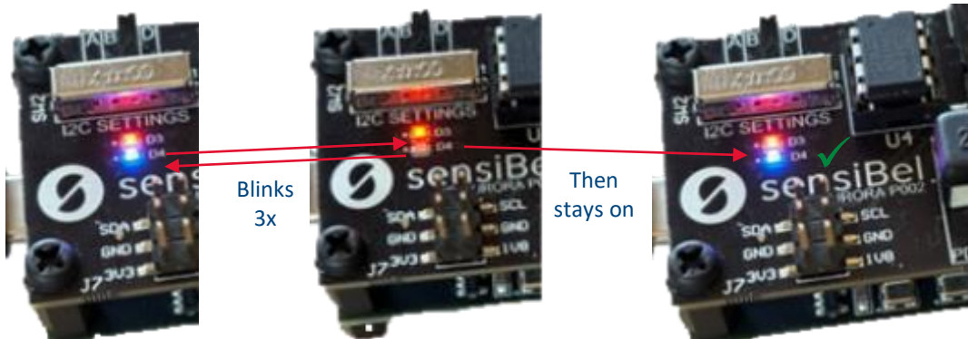
Figure 15. LED sequence for successful I2C write
